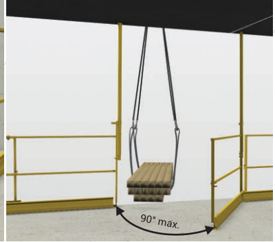
Open the gate fence to a maximum of a 90° angle.
