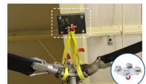
The Type ALP (Adjustable Lifting Point) is Lindapter's standard rigging and lifting solution that safely support loads up to 3.3 tons (6.6 kip) with a +/- 18° lift angle from the supporting steel.
