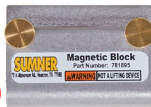
SU781895: Magnetic holders. Great for layout work, super torch guide (3 Per set)
