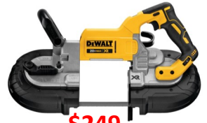
DTDCS374B: Deep Cut Band Saw Cuts up to 5" x 4-3/4" rectangular and 4" round.
