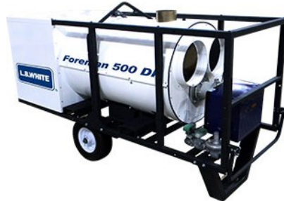
LB White FOREMAN 500 Indirect-Fired Heater LBFOREMAN500: 500,000 BTU/H output, Diesel fired, 42 Gal / 11 Hr operating time, 2 1/2" Outlets
