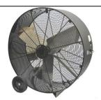
TPIPB-36-D 36" Portable Blower Fan 120V, 1/3 Hp, 2 speed motor, single phase, 6,500 CFM
