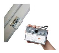
GU10600: 2-Way Universal Standing Seam Roof Clamp. Temporary anchor for use with retractable lifelines . Personal Fall Arrest/Restraint. For all applications: worker weight capacity range (including all clothing, tools, and equipment) is 130-420 lbs.
