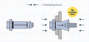
Working closely with Structural Engineers & Steel Fabricators, Lindapter identified the need for the larger M16 & M20 (5/8" & 3/4") Hollo-Bolts to have an increased clamping force suitable for higher strength structural connections. Research & Development led to the invention of the patented 5-part design, optimized for superior performance.
