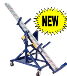
CT513: Elevator Conduit Cart. Tilt allows for easy access into and out of elevators, 500# capacity, Holds standard 10' lengths, fits through 36" doorways. NEW PRODUCT!!!
