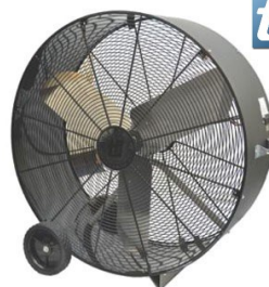
TPPB-36-D 36" Portable Blower Fan 120V, 1/3 Hp, 2 speed motor, single phase, 6,500 CFM.
