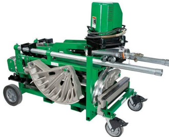
GR881-MBT: Mobile Bending Table. Locking swivel wheels, Fork pockets for fork truck, Vice chain to hold conduit. Stores shoes and saddles when not in use.
