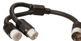
COL01920-00-08: Y adapter for temp power cords. 125/250 Volt AC, 3 pole
