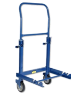
CT504: Reel Cart. 300lb capacity, holds reels of cable up to 20" wide and 40" diameter
