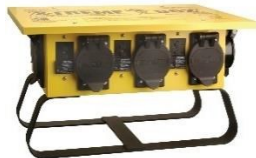
COL01970-3R-02: Temp Power Distribution Spider Box. (6) 20A GFCI and circuit breaker protected NEMA 5-20 straight blade receptacles with covers
