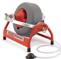
K3800 Drain Cleaner For 3/4" to 4" Drain Lines. Motor automatically gears down when cable hits blockage. Motor: 1/12 HP, 240RPM Line Capacity: 3/4" to 4" pipe Up to 100 ft Item #:.....RI53117
