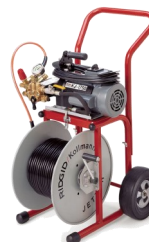
KJ-1750SC Water Jet Jetter provides actual working pressure of 1750 psi to blast through sludge, soap and grease blockages. 1 1/4" to 4" lines. Pulse Thrusts propel hose down the line. Motor: Line Capacity: 1 1/4" to 4" lines Water Pressure: 1750 psi/1.4 gpm Line Capacity: 100' x 3/16" trap hose Item #:.....RI67332
