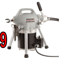
K6200 Drain Cleaner Drum machine cleans sewers and drains up to 6 in. diameter and up to 200 ft long. Motor: 4/10 HP, 285RPM Line Capacity: 3" - 6" pipe Up to 200 ft Item #:.....RI95732
